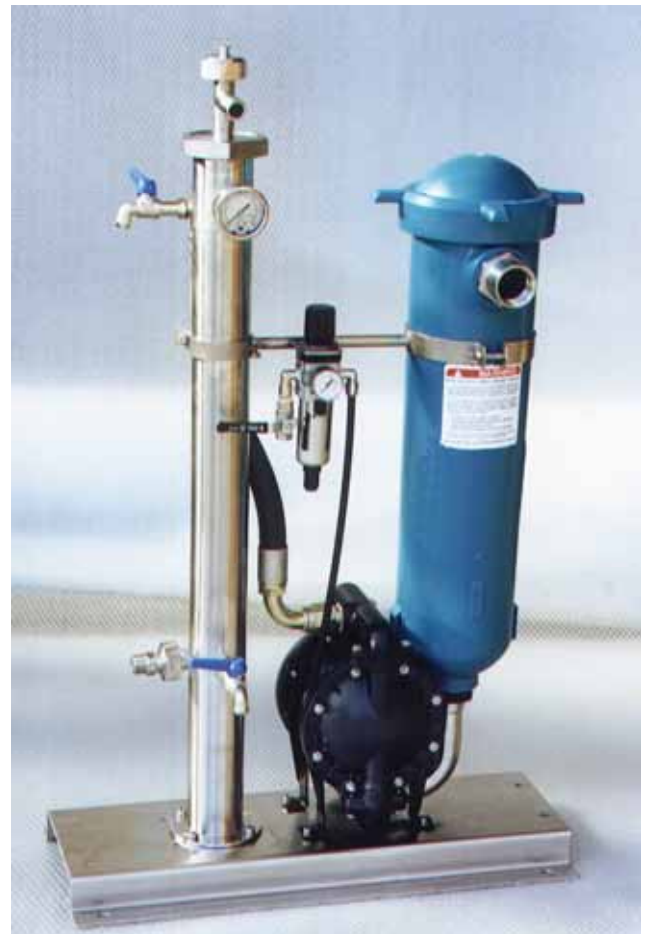
Small Oily Water Treatment Module
