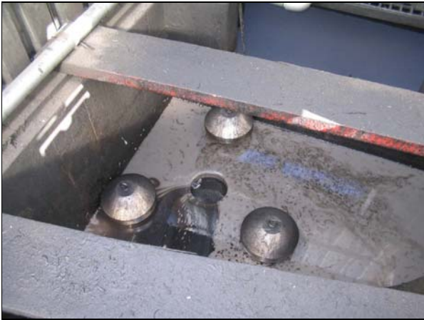
Above: Ultraspin skimmer operating in pit at a coal mine
