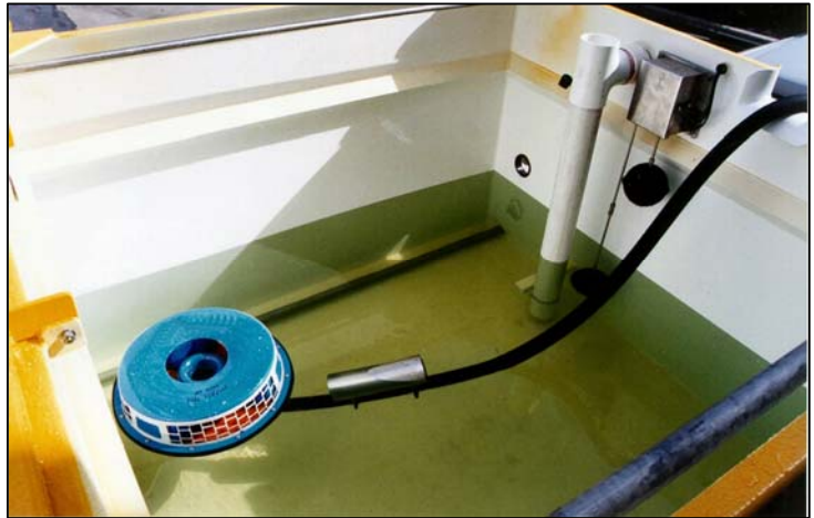
Above: Ultraspin S1 skimmer operating in a small pit
